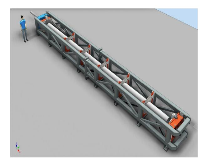
Test rig for pipes; Proportional Pressing clamping style. It has two reaction columns with sector to setting up maximum pipe length. Reaction bridge is moved by hydraulic command.
